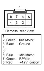
Do **Not u**se this idle control if coil resistance is less than 6 ohm !!!
